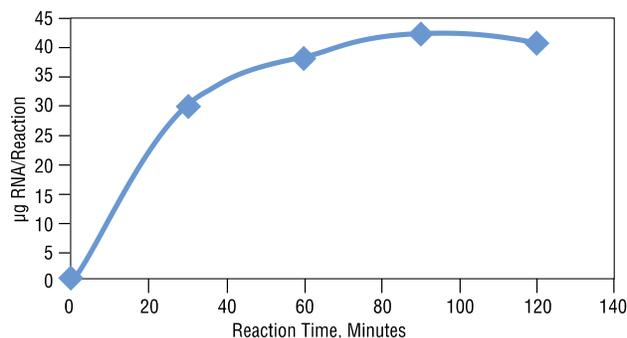
*Reactions were incubated at 37°C in a thermocycler. Transcripts were purified by spin columns and quantified on a NanoDrop Spectrophotometer.*
