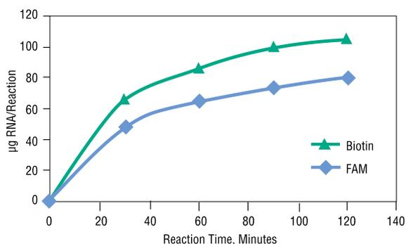
Reactions were incubated at 37°C in a thermocycler. Transcripts were purified by spin columns and quantified on a NanoDrop Spectrophotometer.
