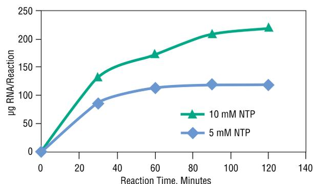
Reactions were incubated at 37°C in a thermocycler. Transcripts were purified by spin columns and quantified on a NanoDrop™ Spectrophotometer.
